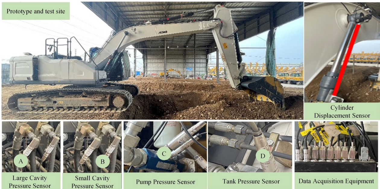
Figure 6 Experiment for operating data acquisition
