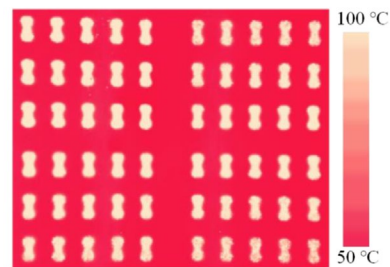
(a) Temperature field data of the eight-shaped part in the fabricating process
