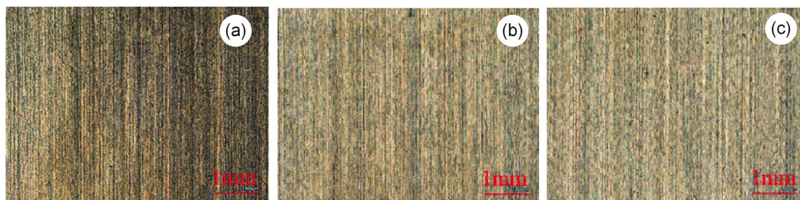
Figure 20 Grinding surface quality: (a) Dry grinding, (b) Flood cooling, and (c) MQL [122]
