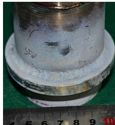
Fig. 7 Photo of welding test sample
