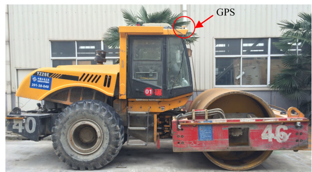
Fig. 3 GPS receiver position on the driver's cab
