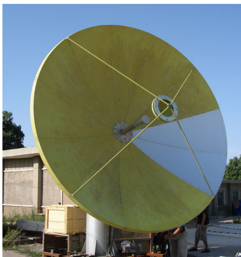
Fig. 5 Panel distribution in reflector surface (front view)
