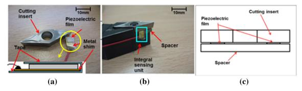
Figure 2 a Composition of the smart cutting tool; b assembly of the tool; c cross section view of the tool
