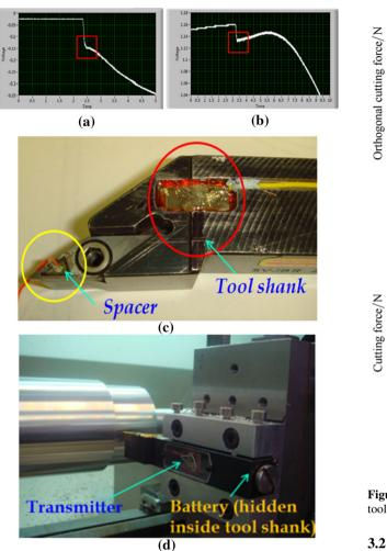
**Figure 4 a** Voltage output from smart tool 1; **b** voltage output from smart tool 2; **c** smart tool 2; **d** cutting trails illustration
