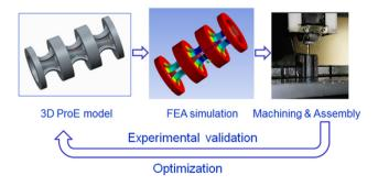
Figure 17 Design of the pull-release tool collet for high speed micro drilling spindles
