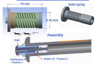
Figure 16 Design layout of an automatic collet for high speed micro milling or micro drilling
