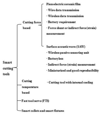
Figure 1 Family schematic of smart cutting tools
