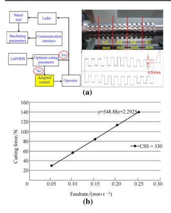
Figure 18 a Adaptive control loop and adaptive smart machining trails on a CNC machine;  $\mathbf{b}$  the relationship between the federate and cutting force
