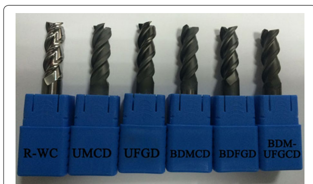
Figure 1 Photographs of the uncoated and different diamond coated milling cutters
