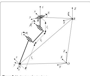
Figure 8 Mechanism of swing leg i
