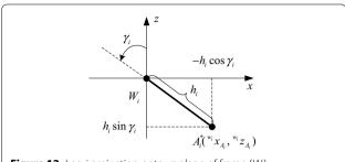
**Figure 12** Leg *i* projection onto xz plane of frame  $\{W_i\}$
