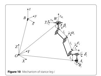
joint and fixed to the body of robot, and the foot reference frame  $\{A_i\}$  is located at the foot of the supporting leg i. The configuration when the leg is fully extended is regarded as the home configuration. In this position, all the joint variables are set to zero.
