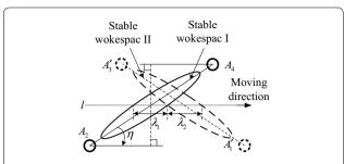
**Figure 17** Two stable workspaces of two adjacent equivalent mechanisms in step forward stages
