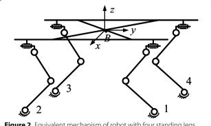
Figure 2 Equivalent mechanism of robot with four standing legs
