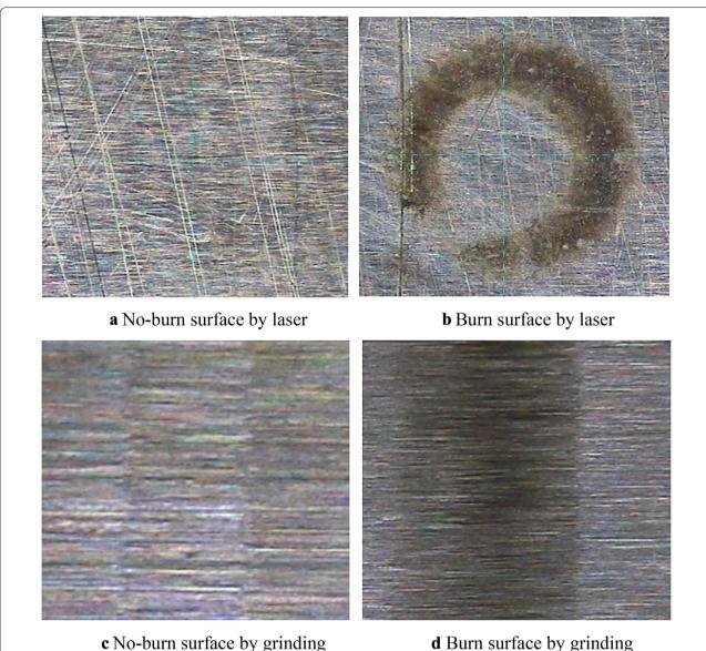
Figure 3 Optical image of laser heating surfaces and grinding surfaces
