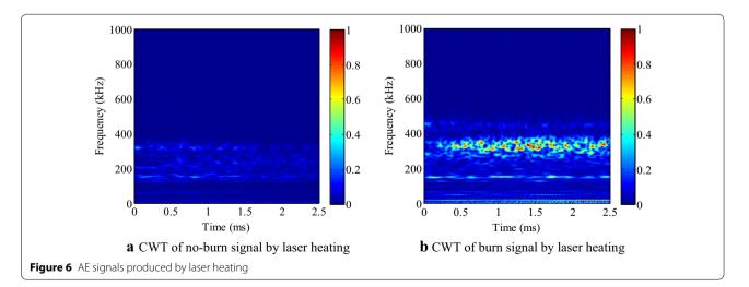
above 100 kHz is relatively low no matter grinding burn happens or not.
