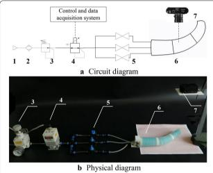
**Figure 9** Schematic of bending angle testing system. 1. Air source; 2. Dryer; 3. Reducing valve; 4. Proportional pressure valve; 5. Shut-off valve; 6. Finger; 7. HDTV camera
