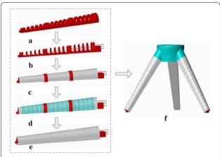
**Figure 5** Fabrication progress of the E-Gripper. **a** The endoskeleton consists of several basic units. **b** Three tubes are embedded into the endoskeleton. **c** One silicon rubber layer is glued around the endoskeleton, and the seal rings are sealed. **d** Circumferential fiber is evenly wound on the surface. **e** A complete soft finger. **f** E-Gripper with three fingers
