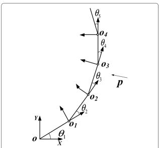
Figure 7 Cartesian coordinate system of a single finger segment
