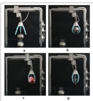
**Figure 15** a Ready for gripping; **b** Gripping an aluminous sphere; **c** Gripping a cloth doll; **d** Gripping a glass bulb
