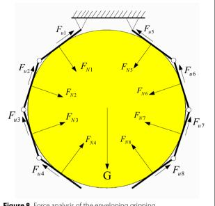
Figure 8 Force analysis of the enveloping gripping
