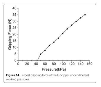
of the cylinder was switched every 10 kPa. Meanwhile, a first-order signal was sent to the proportional pressure valve 10 to increase the pressure slowly until the sphere separated from the gripper and moved downward. The data of the tension sensor were acquired by computer in real time.
