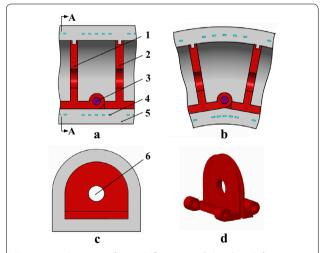
**Figure 1** a Structure of a single finger joint; **b** Bending deformation of the finger joint during air charging; **c** A–A section view; **d** Three-dimensional view of an endoskeleton unit. 1. Endoskeleton unit 1; 2. Endoskeleton unit 2; 3. Hinge; 4. Fiber; 5. Silicon rubber; 6. Flow channel
