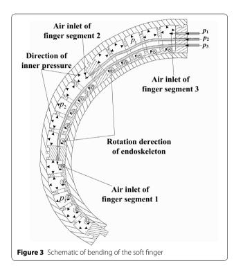
series. The finger joint can rotate from  $-45^{\circ}$  to  $180^{\circ}$  at the hinge joints. To increase the operation efficiency and realize a greater number of postures, the entire finger is divided into three independent finger segments that can be independently pressurized using different air pressures to control the bending angle.
