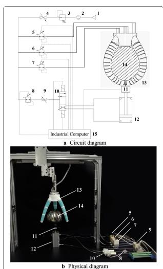
**Figure 13** Gripping force testing circuit. 1. Air source; 2. Dryer; 3. Reducing valve; 4. Shut-off valve; 5, 6, 7, 8. Proportional pressure valve; 9. Throttle valve; 10. Solenoid directional valve; 11. Tension sensor; 12. Cylinder; 13. E-Gripper; 14. Sphere; 15. Computer
