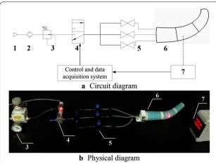
**Figure 11** Schematic of response time testing system. 1. Air source; 2. Dryer; 3. Reducing valve; 4. Solenoid directional valve; 5. Shut-off valve; 6. Finger; 7. Laser displacement sensor
