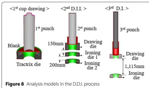
Figure 8 Analysis models in the D.D.I. process
