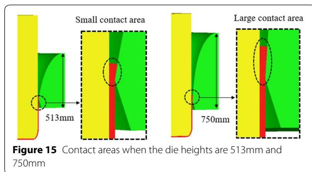
575–600 mm), and fluctuations of the forming load were observed in the transition range (500–650 mm). After then (650–750 mm), the larger contact area allowed to increase the forming load as shown in Figure 15.
