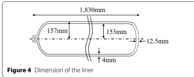
**Figure 4** Dimension of the liner
