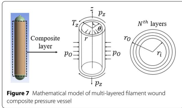
**Figure 7** Mathematical model of multi-layered filament wound composite pressure vessel
