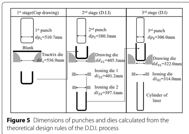
**Figure 5** Dimensions of punches and dies calculated from the theoretical design rules of the D.D.I. process
