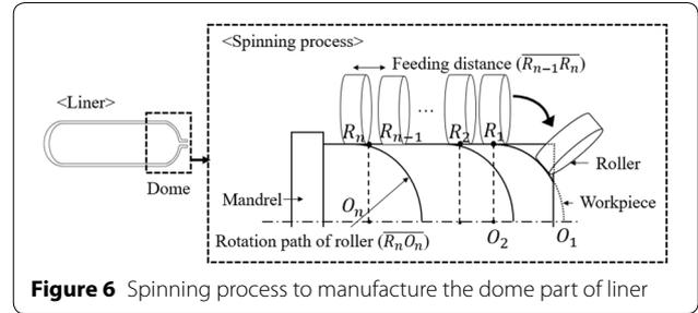
**Figure 6** Spinning process to manufacture the dome part of liner
