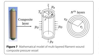
$$\frac{\sigma_1^2}{X^2} + \frac{\sigma_2^2}{Y^2} + \frac{\sigma_3^2}{Z^2} - \sigma_1 \sigma_2 \left( \frac{1}{X^2} + \frac{1}{Y^2} - \frac{1}{Z^2} \right) - \sigma_1 \sigma_3 \left( \frac{1}{X^2} - \frac{1}{Y^2} + \frac{1}{Z^2} \right)
