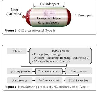
a hot spinning process for dome part, a filament winding process to laminate the composite layers on cylinder part to endure the inner pressure, and a curing process to reinforce adhesive strength between composite layers [8].
