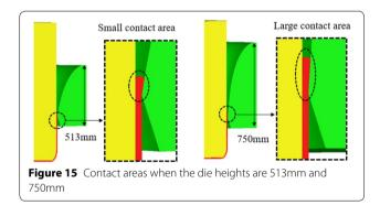
575–600 mm), and fluctuations of the forming load were observed in the transition range (500–650 mm). After then (650–750 mm), the larger contact area allowed to increase the forming load as shown in Figure 15.
