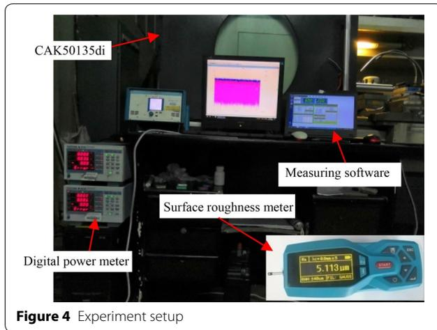
Figure 4 Experiment setup
