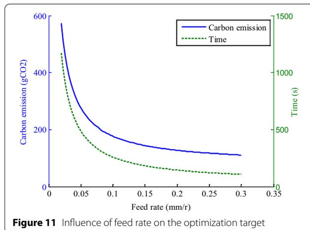
Figure 11 Influence of feed rate on the optimization target
