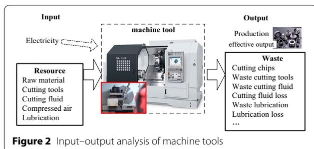
Figure 2 Input–output analysis of machine tools
