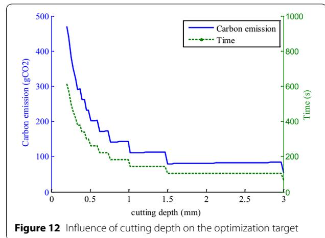
Figure 12 Influence of cutting depth on the optimization target
