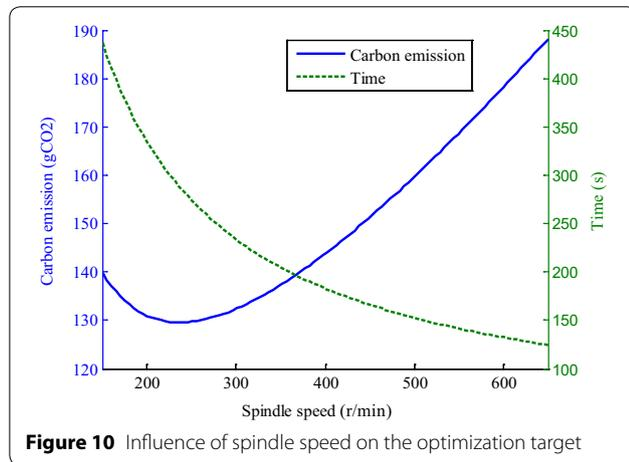
Figure 10 Influence of spindle speed on the optimization target
