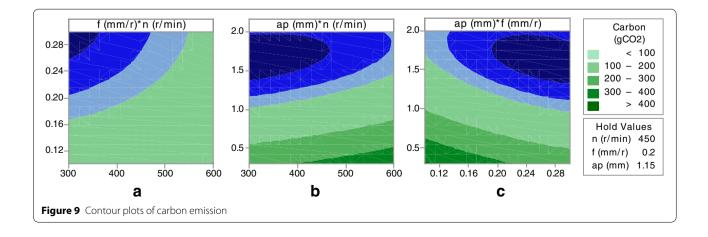
of the cutting depth on the carbon emissions are more significant than those of the spindle speed on the carbon emission (Figure 9(a)), whereas the effects of the cutting depth on the carbon emissions are more significant than the feed rate on the carbon emissions (Figure 9(b)), This is also consistent with the analysis results in Section 5.2.
