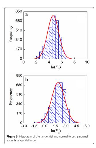
lognormal distribution. Meanwhile, the mean and standard deviation of each cutter's forces were obtained. Based on the distribution form, the mean and the standard deviation, the random forces on each cutter can be generated by using the Latin Hypercube Sampling method.
