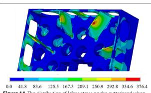
**Figure 14** The distribution of Mises stress on the cutterhead when t = 19.80 s (unit: MPa)
