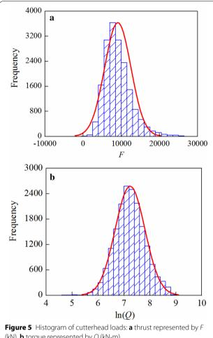
(kN), **b** torque represented by Q (kN·m)
