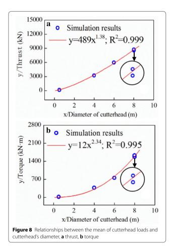
model for the mean of cutterhead loads was formulated as
