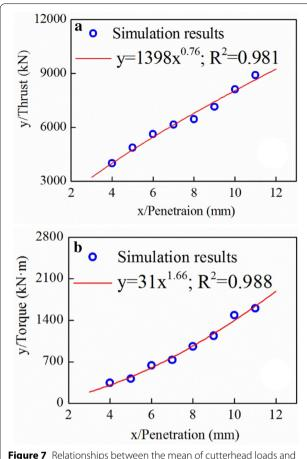
**Figure 7** Relationships between the mean of cutterhead loads and penetration, **a** thrust, **b** torque
