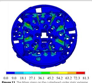
**Figure 11** The Mises stress on the cutterhead under static extreme loads (unit: MPa)
