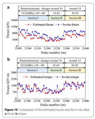
value shows a good agreement with the measured data, and the mean of the relative error is 17.10%.
