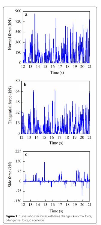
a high dispersion and the peak rock-breaking forces occur in a very low frequency.
