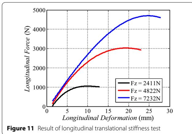
Figure 11 Result of longitudinal translational stiffness test
