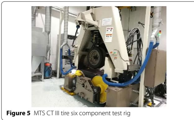
Figure 5 MTS CT III tire six component test rig
