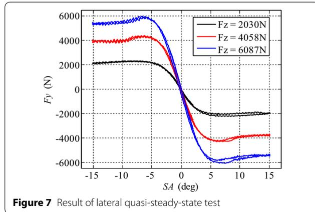
**Figure 7** Result of lateral quasi-steady-state test
