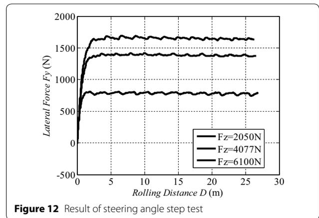
Figure 12 Result of steering angle step test
