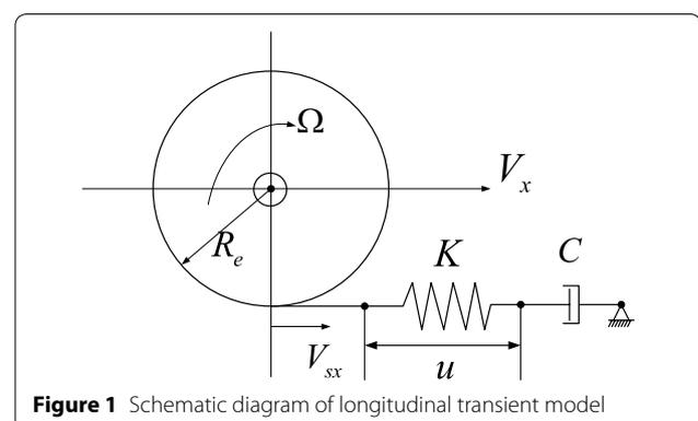
Figure 1 Schematic diagram of longitudinal transient model
