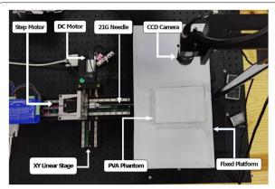
Figure 4 Experimental testbed for needle insertion procedures
