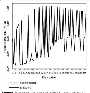
**Figure 4** Experimental and predicted cylinder pressure values of 91 test data points
