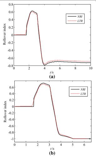
**Figure 3** Comparison between *LTR* and *NRI* in Fishhook maneuver: (a) u = 55 km/h; (b) u = 65 km/h.
