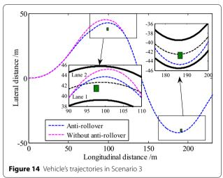
driving condition. The front wheel steering angle output by the motion planning strategy with active anti rollover ability a slightly less than that without active anti rollover ability. From the results in Figure 11, it can be illustrated that the proposed strategy can avoid obstacles smoothly and reduce the vehicle rollover risk during cornering.
