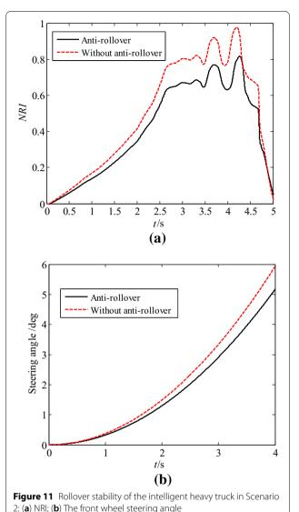
Scenario 2: Obstacle avoidance on curved road. As shown in Figure 9, the ego vehicle is travelling on Lane 1 at an initial speed of 80 km/h, and the vehicle 1 is travelling on Lane 2 at a constant speed of 80 km/h. There is a fixed obstacle of 1 m in length and width in the curve part on Lane 1. The ego vehicle needs to make an emergency change to Lane 2, and reduce the speed in order not to collide with vehicle 1 on Lane 2.
