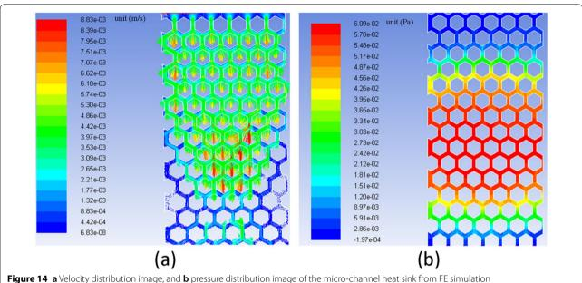
Figure 14 a Velocity distribution image, and b pressure distribution image of the micro-channel heat sink from FE simulation
