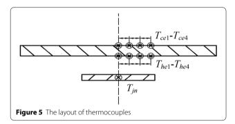
Bakelite insulation, experimental measurement temperature will be lower than the actual temperature. A pair of thermocouple is placed at the center of every heating rod to measure the simulated LED chip junction temperature. In order to eliminate the clearance between the heating module and heat sink, a thin layer of thermal conductive silicone was evenly coated on the surface of the aluminium block.
