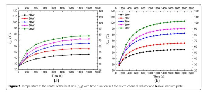
then remains steady not until 20 min. Figure 7b shows that the temperature increases all the time, and cannot get a balance in 30 min. The fast response of micro-channel radiator is attributed to the phase change heat dissipation. Generally, the time to reach thermal balance is to measure the start-up performance of a radiator. Thus, the developed micro-channel radiator has a great start-up heat transfer performance.
