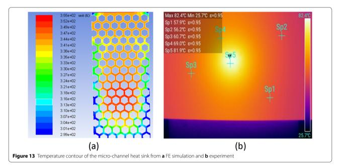
the specimen under the input power of 90 W is photographed using infrared imager as shown in Figure 13(b). Sp1 to sp5 refer to 5 typical measurement points, while  $\varepsilon$  is emissivity. The highest temperature from simulation is (355-273.15)=81.85 °C, corresponding to the 82.4 °C in the experiment. The lowest temperature is (299-273.15)=25.85 °C, corresponding to the 25.7 °C in the experiment. Upon the
