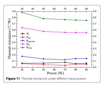
to further reduce the junction temperature of the chip, thermal convective resistance of the surface of the microchannel radiator should be further reduced by the optimization of surface structure.
