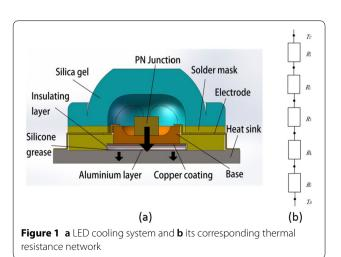
$$R_{Total} = R_{in} + R_{out} = R_1 + R_2 + R_3 + R_4 + R_5,$$
