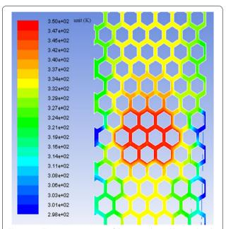
**Figure 15** Temperature contour of the micro-channel heat sink with the best combination (*A4B1C1D4*)
