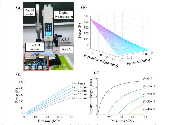
**Figure 5** Output characteristics of the RSPA: (a) Test system for the RSPA, (b) The performance parameter relationships between output force, expansion height and pressure of the RSPA, (c) The relationship between output force and pressure of the RSPA at different expansion heights, (d) The relationship between expansion height and pressure of the RSPA at different output forces
