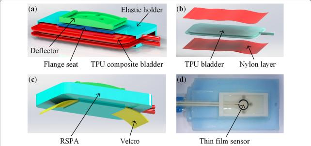
**Figure 1** Structure of the RSPA: (a) Cross-section diagram of the RSPA, (b) Two nylon layers are laminated onto the surface of the TPU composite bladder, (c) The Velcro passes through the bottom channel of the RSPA to bond the RSPA to the wearable carrier, (d) A thin film sensor is installed in the center of the deflector
