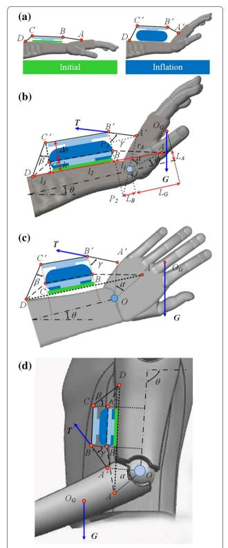
**Figure 4** Analysis of rehabilitation motion: (a) Wrist posture changes under the action of the RSPA, (b) Illustration of wrist extension, (c) Illustration of wrist ulnar deviation, (d) Illustration of elbow flexion
