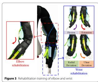
to arrange four RSPAs around the wrist joint to drive the wrist to perform rehabilitation movements, as shown in Figure 3.
