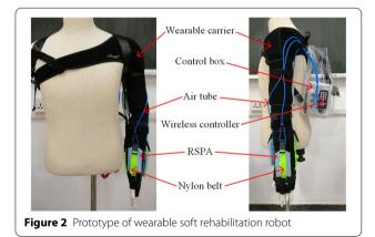
and elastic. The tightness of the wearable carrier can be adjusted according to the needs of the patients to ensure comfort.
