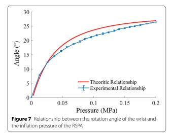
between the inflation pressure of the RSPA and the rotation angle of the wrist fitted onto the experimental measurements is marked by a blue line in Figure 7, and the relationship curve between the inflation pressure of the RSPA and the rotation angle of the wrist, which is deduced by motion theory, is marked by a red line in Figure 7.
