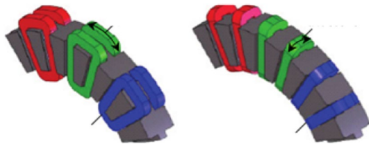
Figure 2 Winding structure of AFPMSM: a Drum and b Toroidal windings
