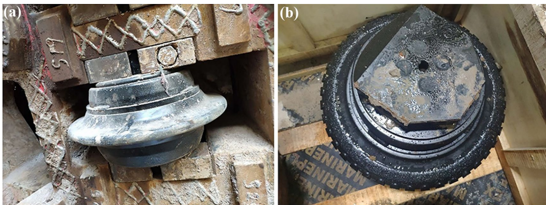
Figure 6 Cutters used in the field: a Disc cutter, and b Wedge tooth cutter
