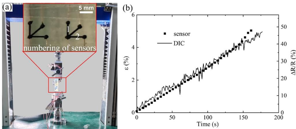
**Figure 8** Calibration of  $GF$  for the printed strain rosette sensor: (a) Specimen with separated strain rosette clamped on the test machine, (b) Strain measured by DIC and the resistance variation recorded by the sensor unit
