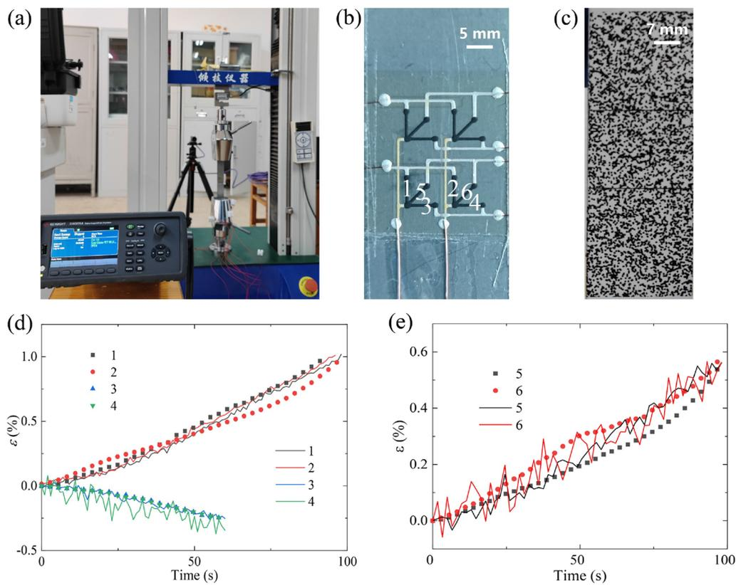
**Figure 9** Strain monitoring for a specimen based on the printed strain rosette sensor array: (a) Testing set up, (b) and (c) Two sides of the specimen attached by the printed strain rosette sensor array and DIC-speckle, (d) and (e) Real-time recording strain data at the six marked branches monitored by the printed strain rosette sensor array and the data extracted from the DIC
