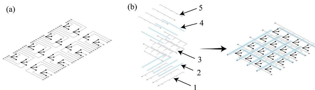
**Figure 1** Circuit layout of (a) traditional circuit layout and (b) developed multilayer design for the strain rosette array composed of  $4 \times 4$  units
