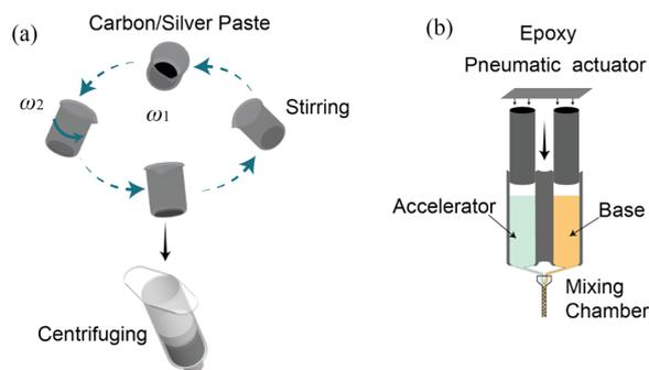
**Figure 6** Preparation for (a) carbon/silver paste and (b) epoxy
