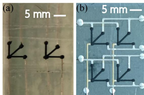
**Figure 7** Samples for the DIW printed (a) separated strain rosettes and (b) arrays with  $2 \times 2$  units
