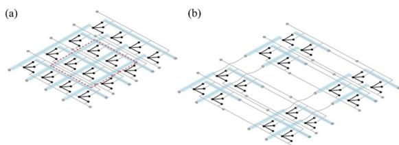
**Figure 5** Two typical strategies for scalable strain rosette sensor array: (a) Through expanding the basic circuit layout, (b) By connecting the electrodes of separated sensor arrays orderly
