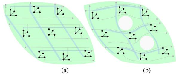
**Figure 4** Adaptability of the strain rosette sensor arrays for arbitrary-shaped (a) simple connected and (b) multi connected domain
