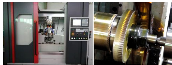
Figure 22 Hobbing experimental platform of the oval gear
