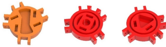
(a) Central node on reflecting surface (b) Boundary node on reflecting surface (c) Node on back surface
