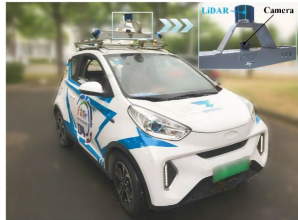
Figure 5 The autonomous vehicle carrying the sensor setup
