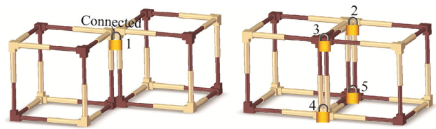
Fig. 4. Connection methods between neighboring two PE-Cubes
