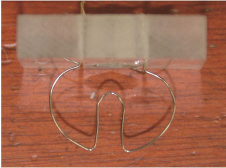
(b) Elastic link mechanism fixed with an acrylic block
