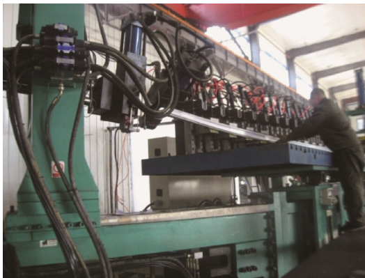
Fig. 8. Profile in three-dimensional stretch bending forming process
