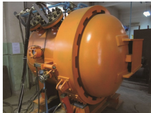
Fig. 2 Hyperbaric welding chamber
