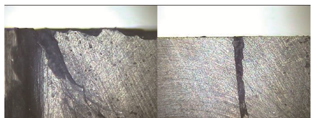
Fig. 10. Cracks of workpiece induced by thermal stress
