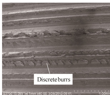
Fig. 9. Discrete burrs formed on the free side of cutting layer of a tooth
