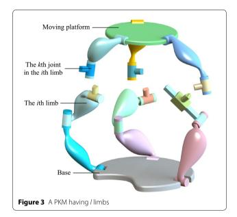
(P)). Because the finite motions of the PKM's moving platform can be obtained as the intersection of those of its limbs, and the finite motions of each limb are the composition of those of all joints in it, following analytical equations can be formulated through describing the finite motions of the PKM, its limbs and joints as finite screws.
