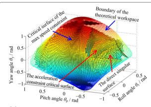
(a) Workspace of the 4-PSS/PS mechanism when  $L_0$ =1000 mm,  $L_1$ =2500 mm,  $L_2$ =1955 mm,  $L_3$ =2500 mm,  $L_4$ =1500 mm
