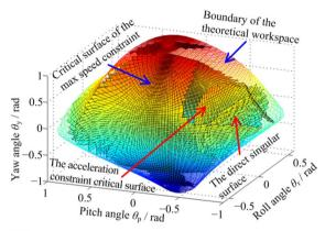
**(b)** Workspace of the 4-PSS/PS mechanism when  $L_0$ =1000 mm,  $L_1$ =2500 mm,  $L_2$ =2040 mm,  $L_3$ =2500 mm,  $L_4$ =1500 mm
