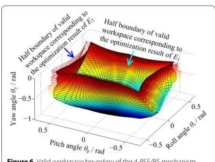
**Figure 6** Valid workspace boundary of the 4-<u>PSS/PS</u> mechanism corresponding to the two optimal mechanism parameter sets
