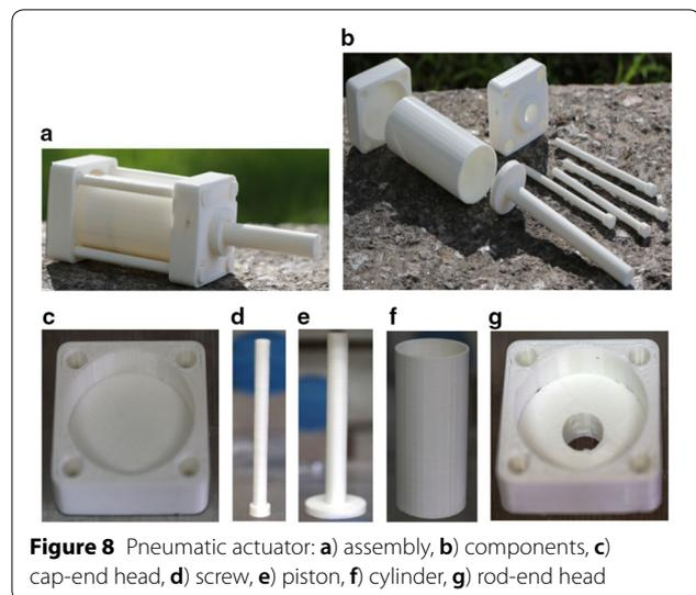
were made. Figure 8 shows the pneumatic actuator components after their fabrication.
