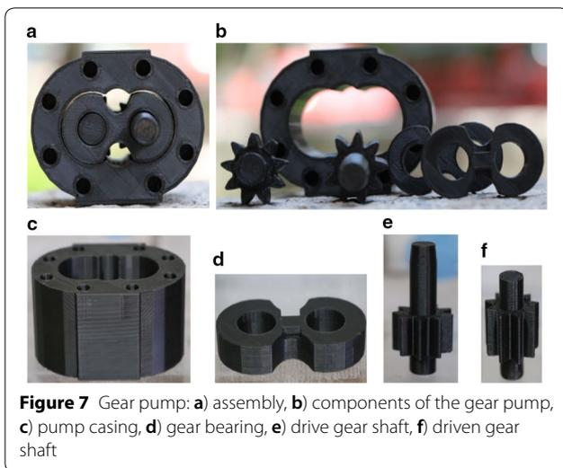
and application of the proposed DfAM strategies. Figure 7 shows the gear pump components after their fabrication.
