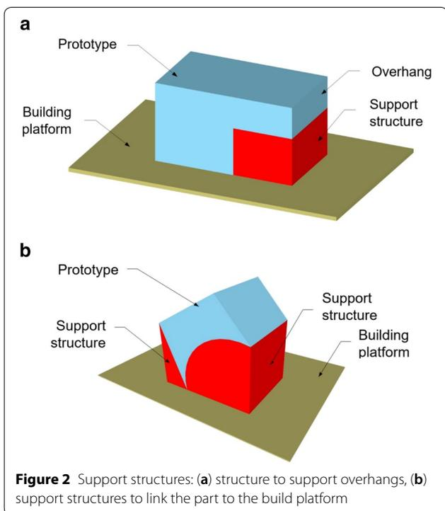
**Figure 2** Support structures: (a) structure to support overhangs, (b) support structures to link the part to the build platform
