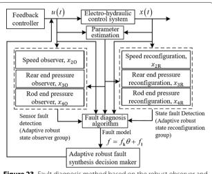
**Figure 23** Fault diagnosis method based on the robust observer and the state reconstruction
