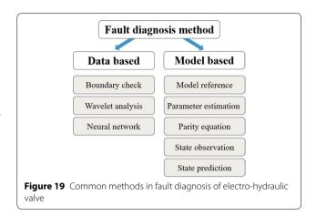
the numerical threshold to monitor the operation states of the valve. Afterwards, the state quantities of the valve are checked to see if they exceed the preset threshold value to diagnose the faults.
