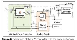
**Figure 8** Schematic of the SLM controller with the switch of power supply
