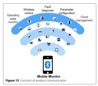
In regard to the demand for wireless communication networks, some enterprises have released products that are integrated with Bluetooth. SUN 7904A24, a proportional cartridge valve, integrates Bluetooth. HAWE RV2S-BT integrates Bluetooth, which makes valves convenient and intelligent to control, monitor and manage. Figure 15 shows what wireless communication can do.
