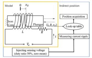
**Figure 3** Schematic of the valve's solenoid and indirect position acquisition method
