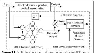
**Figure 21** Fault diagnosis method based on a two-stage RBF neural network
