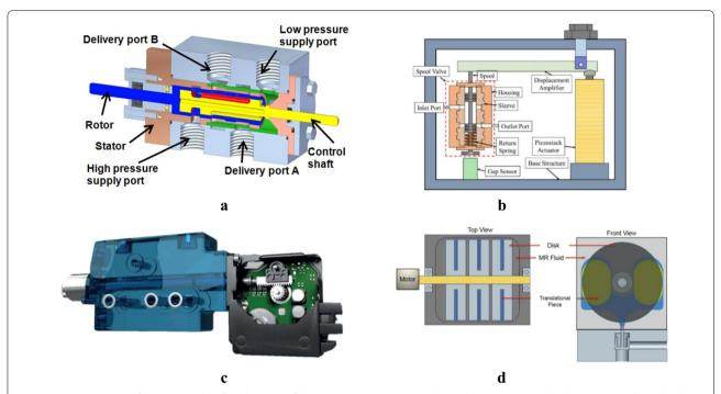
Figure 7 (a) Schematic of the rotary valve; (b) Schematic of the piezoelectric actuator valves; (c) Electromechanical valve actuator; (d) Stacked valve configuration of the electronic control valve (ECV)
