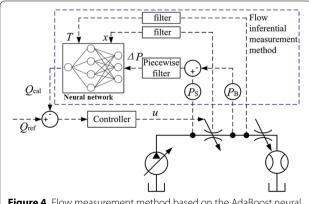
**Figure 4** Flow measurement method based on the AdaBoost neural network
