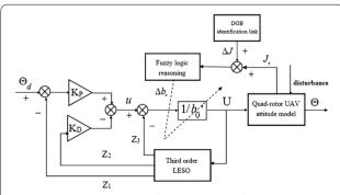
**Figure 3** Adaptive controller of attitude tracking for the quad-rotor based on LADRC
