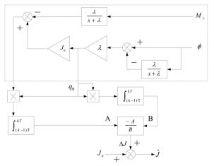
**Figure 2** Diagram of the identification of rotational inertia based on the DOB
