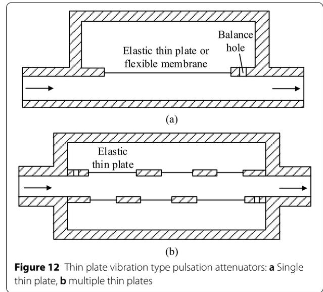
**Figure 12** Thin plate vibration type pulsation attenuators: **a** Single thin plate, **b** multiple thin plates
