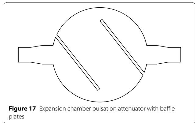
**Figure 17** Expansion chamber pulsation attenuator with baffle plates
