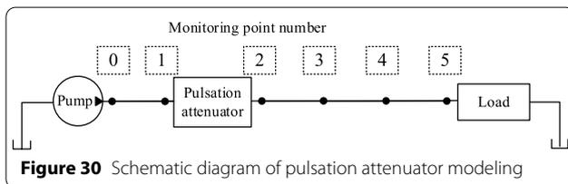
**Figure 30** Schematic diagram of pulsation attenuator modeling
