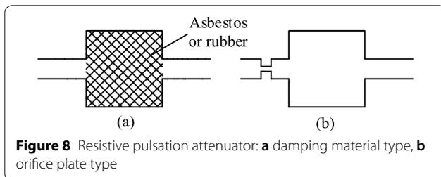
principles: resistive, reactive, and composite pulsation attenuators [41].
