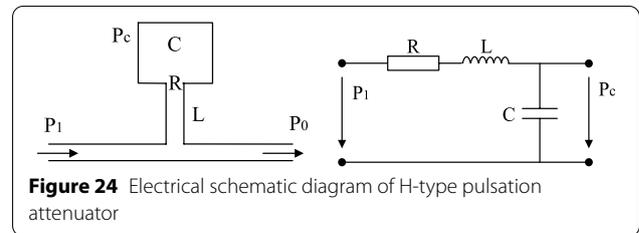
**Figure 24** Electrical schematic diagram of H-type pulsation attenuator
