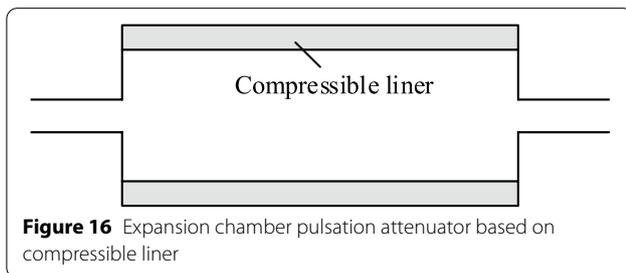
**Figure 16** Expansion chamber pulsation attenuator based on compressible liner
