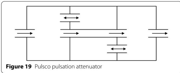
Figure 19 Pulsco pulsation attenuator
