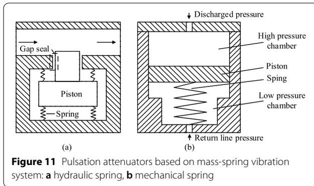
**Figure 11** Pulsation attenuators based on mass-spring vibration system: **a** hydraulic spring, **b** mechanical spring
