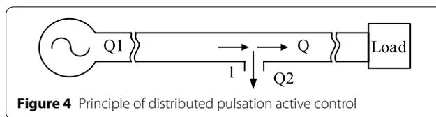
Figure 4 Principle of distributed pulsation active control
