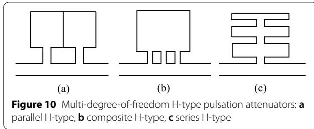
**Figure 10** Multi-degree-of-freedom H-type pulsation attenuators: **a** parallel H-type, **b** composite H-type, **c** series H-type
