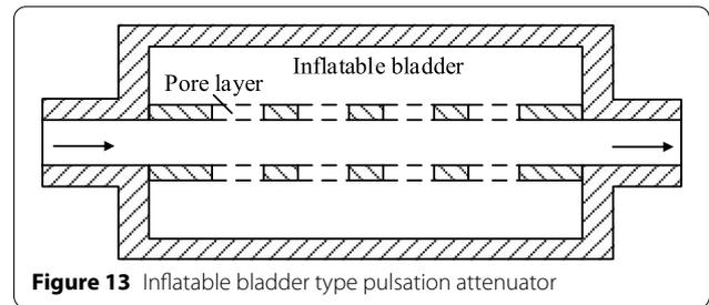
**Figure 13** Inflatable bladder type pulsation attenuator
