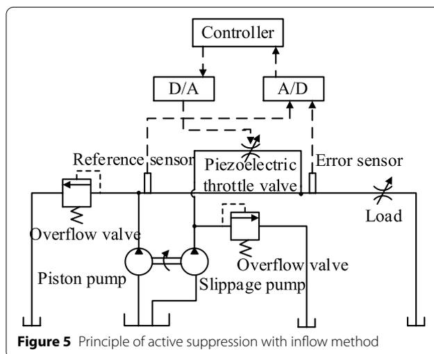
Figure 5 Principle of active suppression with inflow method
