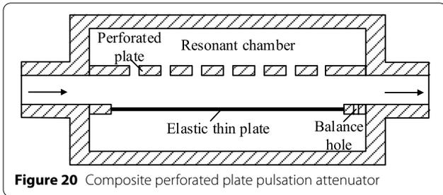
Figure 20 Composite perforated plate pulsation attenuator
