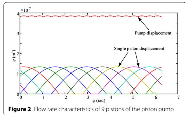
**Figure 2** Flow rate characteristics of 9 pistons of the piston pump
