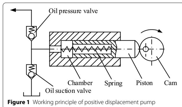
**Figure 1** Working principle of positive displacement pump
