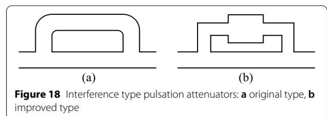
**Figure 18** Interference type pulsation attenuators: **a** original type, **b** improved type
