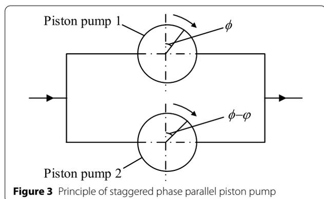
Figure 3 Principle of staggered phase parallel piston pump
