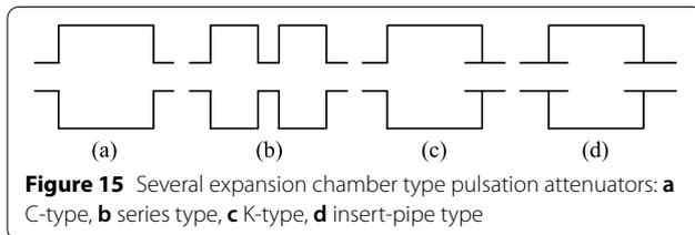
**Figure 15** Several expansion chamber type pulsation attenuators: **a** C-type, **b** series type, **c** K-type, **d** insert-pipe type
