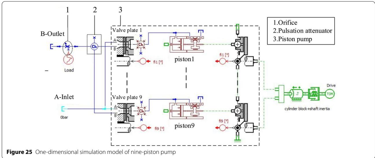
Figure 25 One-dimensional simulation model of nine-piston pump
