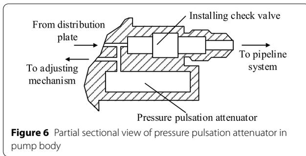
**Figure 6** Partial sectional view of pressure pulsation attenuator in pump body
