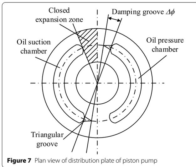
**Figure 7** Plan view of distribution plate of piston pump
