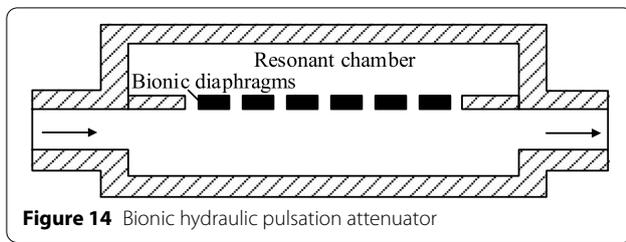
**Figure 14** Bionic hydraulic pulsation attenuator
