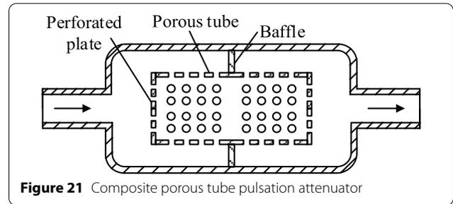
Figure 21 Composite porous tube pulsation attenuator
