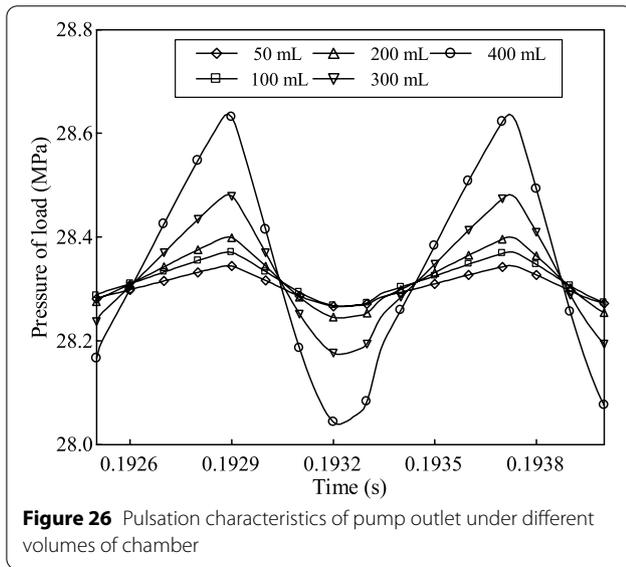
Figure 26 Pulsation characteristics of pump outlet under different volumes of chamber
