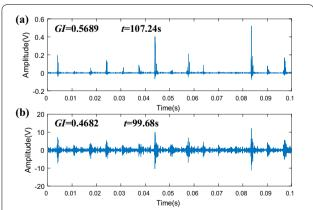
**Figure 17** Waveforms of **a** the feature obtained by the original TM method and **b** the optimal target mode obtained by the PSO-VMD method for the signal in Figure 15
