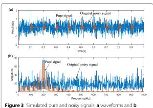
**Figure 3** Simulated pure and noisy signals: **a** waveforms and **b** spectra
