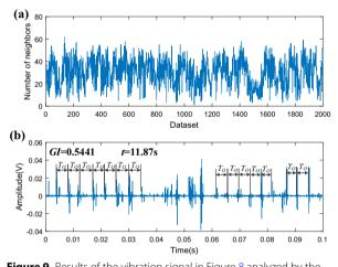
**Figure 9** Results of the vibration signal in Figure 8 analyzed by the proposed method: **a** the reallocated neighbor numbers by the TN algorithm and **b** the waveform of the synthetic TM feature
