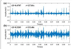
**Figure 10** Waveforms of **a** the feature obtained by the original TM method and **b** the optimal target mode obtained by the PSO-VMD method for the signal in Figure 8
