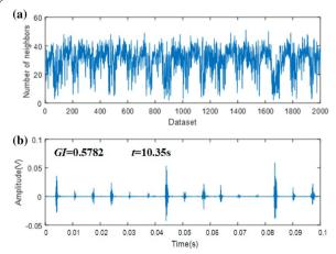
**Figure 16** Results of the acoustic signal in Figure 15 analyzed by the proposed method: **a** the reallocated neighbor numbers by the TN algorithm and **b** the waveform of the synthetic TM feature
