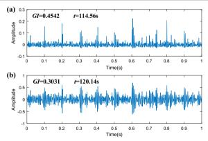
**Figure 7** Waveforms of **a** the feature obtained by the original TM method and **b** the optimal target mode obtained by the PSO-VMD method for the signal in Figure 3
