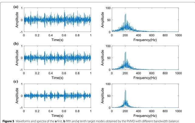
Figure 5 Waveforms and spectra of the **a** first, **b** fifth and **c** tenth target modes obtained by the RVMD with different bandwidth balance parameters for the signal in Figure 3
