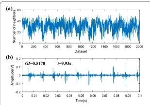
Figure 13 Results of the acoustic signal in Figure 12 analyzed by the proposed method: a the reallocated neighbor numbers by the TN algorithm and **b** the waveform of the synthetic TM feature
