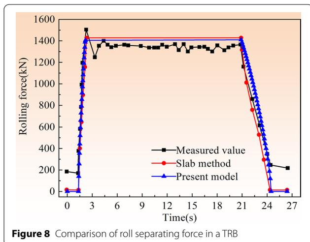
Figure 8 Comparison of roll separating force in a TRB
