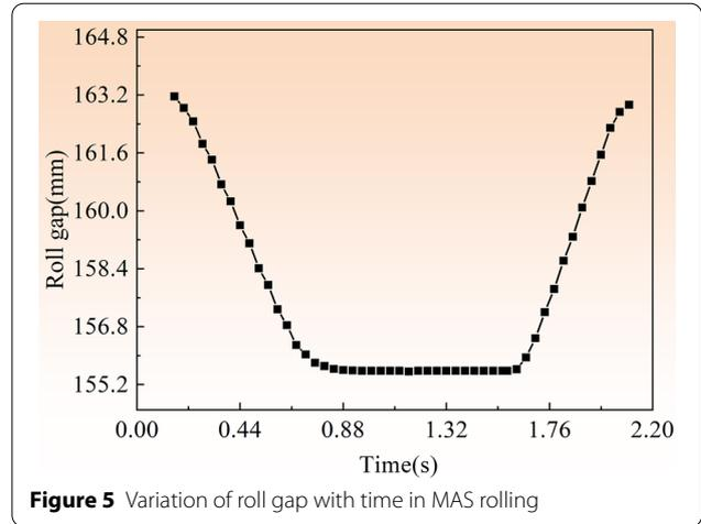
Figure 5 Variation of roll gap with time in MAS rolling
