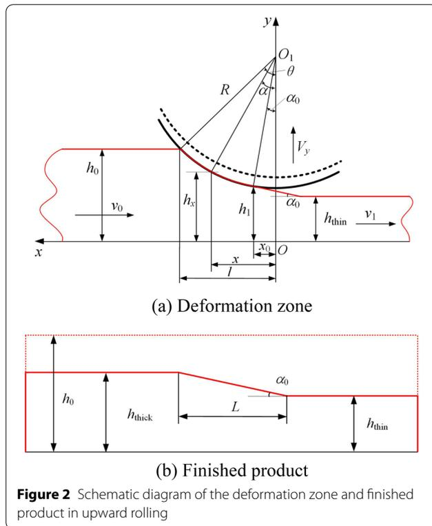
**Figure 2** Schematic diagram of the deformation zone and finished product in upward rolling
