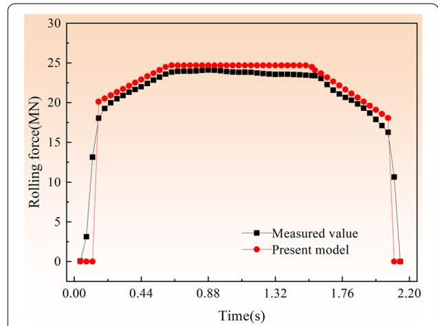
Figure 6 Comparison of roll separating force for theoretical and measured values in MAS rolling
