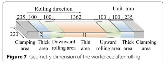
Figure 7 Geometry dimension of the workpiece after rolling
