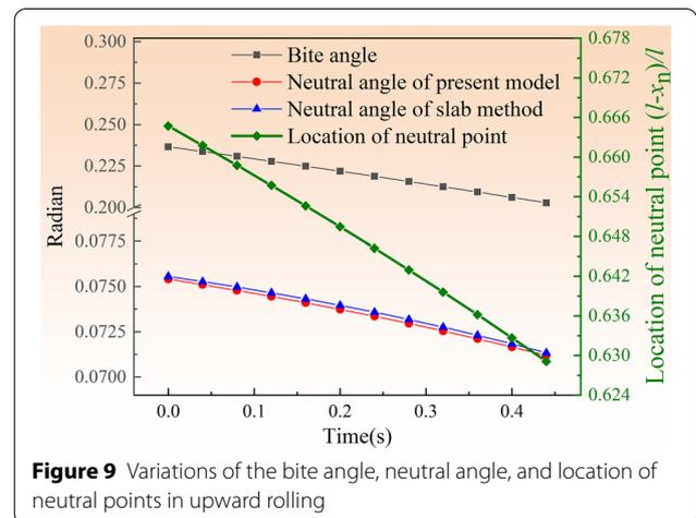
Figure 9 Variations of the bite angle, neutral angle, and location of neutral points in upward rolling
