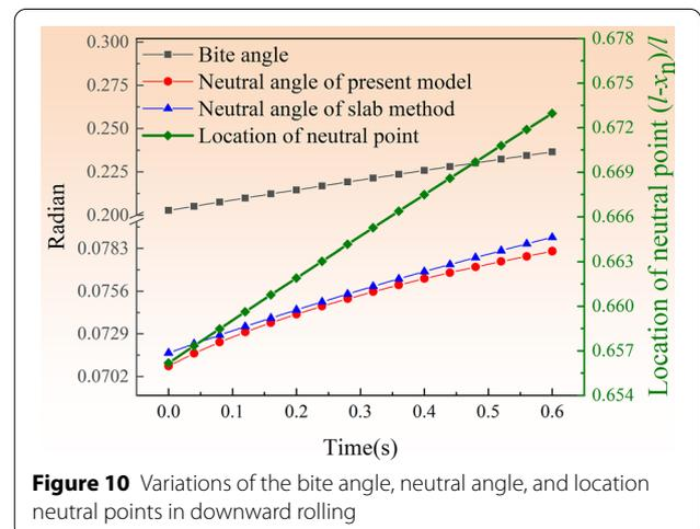
Figure 10 Variations of the bite angle, neutral angle, and location neutral points in downward rolling
