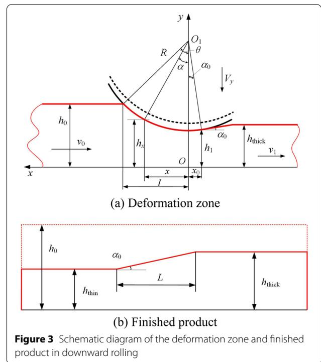
**Figure 3** Schematic diagram of the deformation zone and finished product in downward rolling
