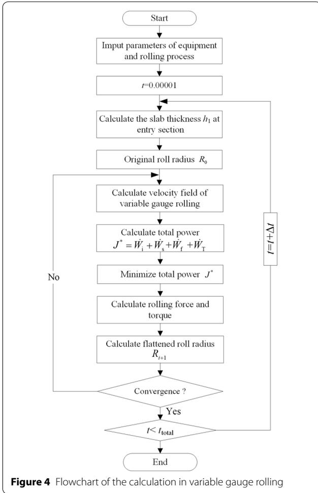
Figure 4 Flowchart of the calculation in variable gauge rolling
